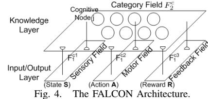
Fig. 4. The FALCON Architecture.
