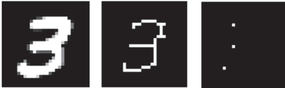
Fig. 8. Original digit image, its skeleton, and the location of its endpoints
