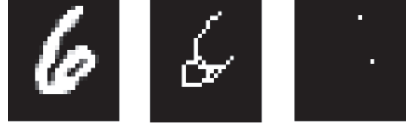
Fig. 9 Spurious endpoint in digit 6.
