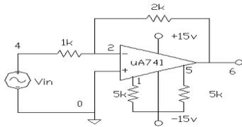
Figure 2.b Negative feedback configuration of  $\mu$ A741.
