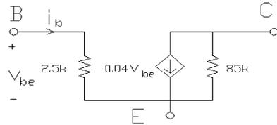
Figure 2.c The small signal model of BJT.
