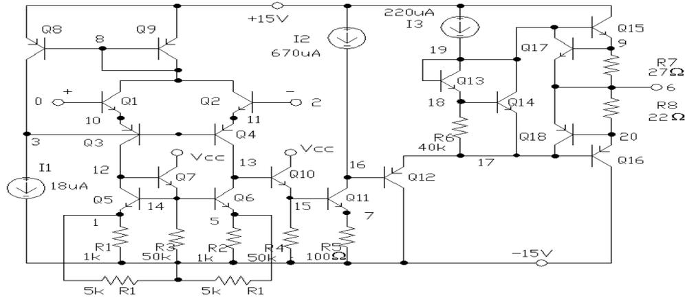
Figure 2.a overall schematic of the Fairchild  $\mu$ A741 operational amplifier.
