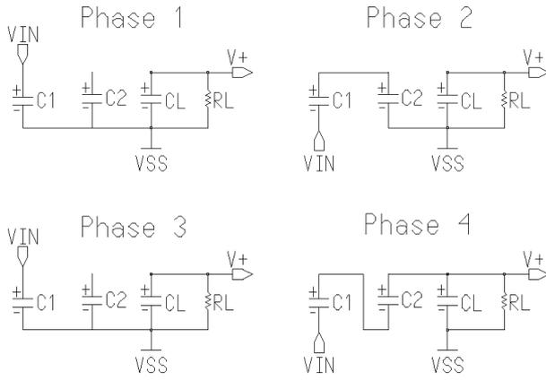
Fig. 7. Equivalent circuits of 2-stage MPVD
