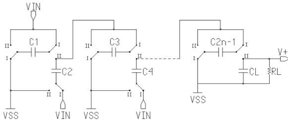
Fig. 3. Two-phase voltage doublers (Makowski charge pump)
