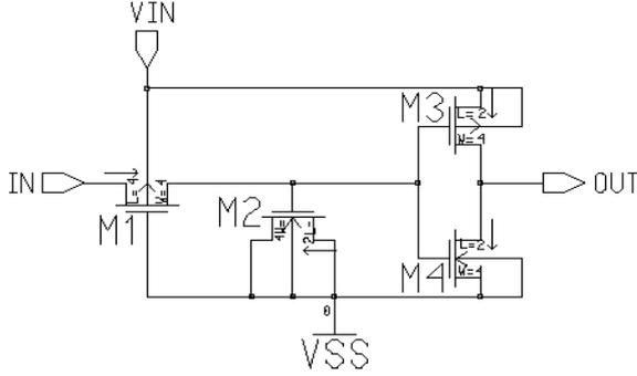
Fig. 10. RC-inverter
