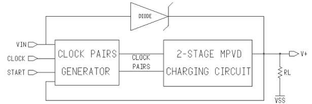
Fig. 5. Diagram of 2-stage MPVD
