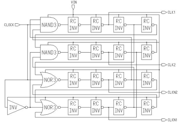
Fig. 9. Non-overlapping clock pairs converter
