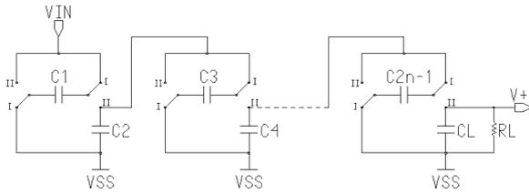
Fig. 2. Two-phase voltage doublers (simply cascaded)
