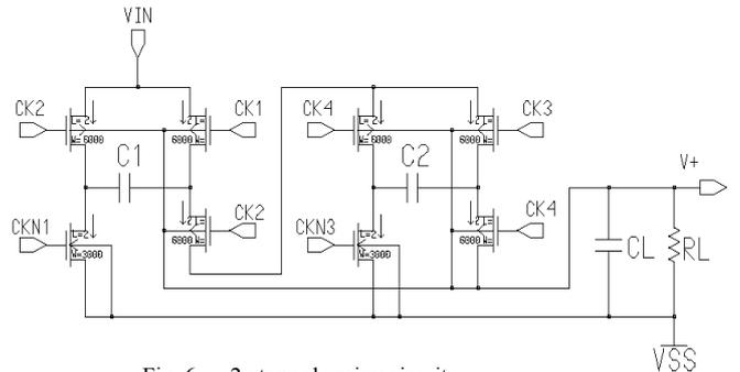
Fig. 6. 2-stage charging circuit
