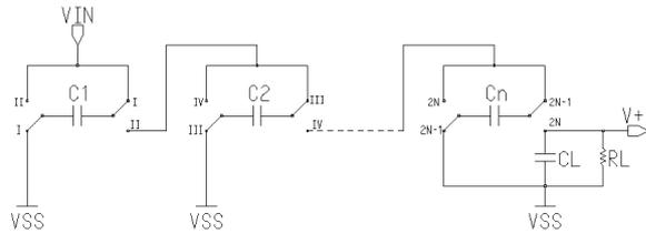
Fig. 4. Multi-phase voltage doublers (MPVD)
